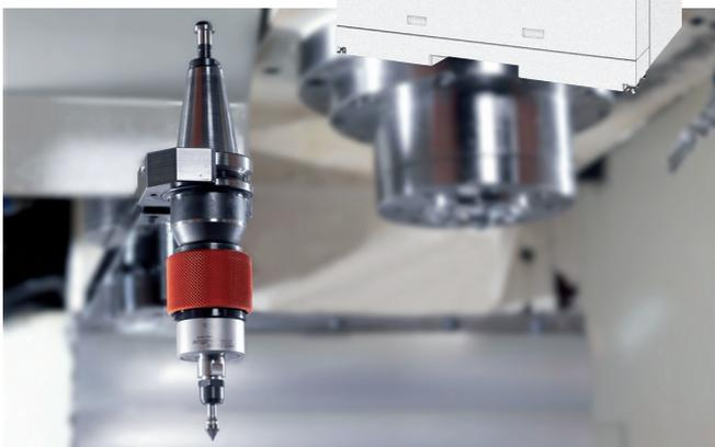
Version with integrated drive spindle in use for workpiece deburring with robot
